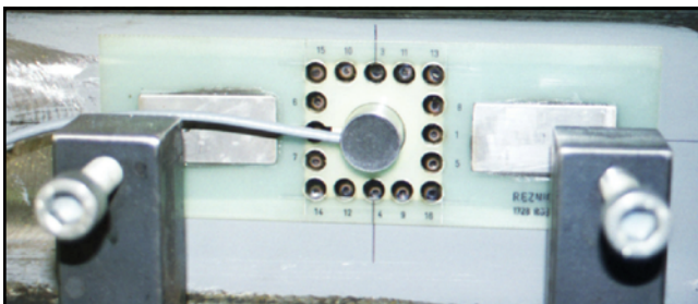
Spot welding of KG-03 Extensometer on a rail
