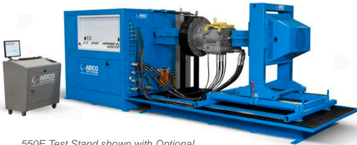
550E Test Stand shown with Optional Output Load Unit, Shift Cart, and Bell Housing Mounting Kit
